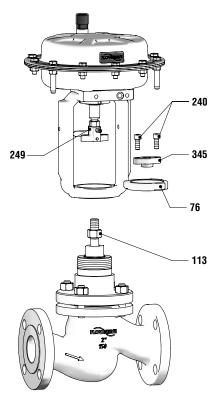
Figure 8: Remove the actuator
