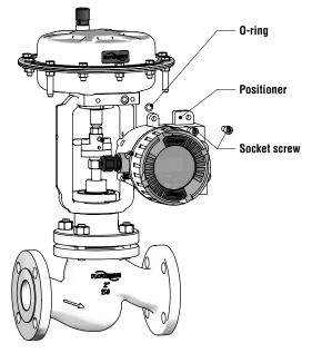
Figure 7: Remove the positioner
