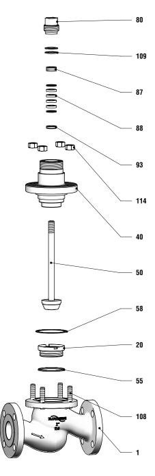
Figure 9: Disassemble / Reassemble the valve
