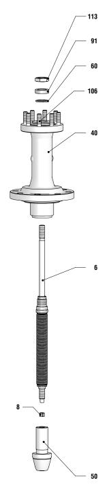
Figure 11: Disassemble / Reassemble the valve with bellows seal assembly for type B design
