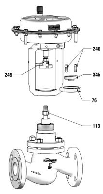
Figure 15: Remove the actuator
