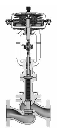
Figure 2: Valtek GS with Bellows Seal Bonnet
