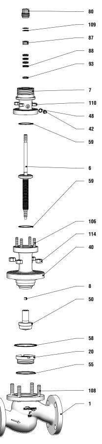
Figure 10: Disassemble / Reassemble the valve with bellows seal assembly for type A designs (Valve parts see Table 13, Page 17)
