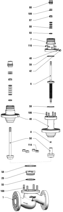
Figure 16: Complete valve parts
