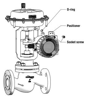
Figure 14: Remove the positioner
