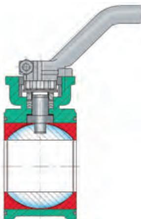
In order to prevent product residues and to prevent the interior from running completely empty, the seat rings filling the cavities enclose the ball and fill the otherwise present cavity.
