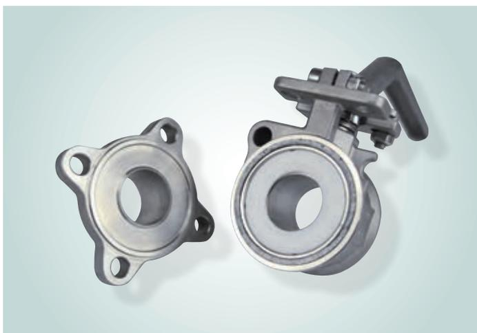
If PTFE sealed valves are exposed to flames in case of fire, this may cause the melting of the sealing materials, which will inevitably result in leakages to the outside and in the bore. In order to be suitable for these requirements, the ball valve DGF is equipped with a special sealing system.
